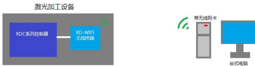
Figure-1 One desk-top computer wireless connection diagram (Configured WIFI network card with USB interface)
