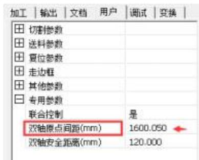
Although the dual laser head hard limit protection has been set, the hard limit is only a guarantee under abnormal conditions. In normal , it should be ensured that the controller has terminated before the hard limit protection occurs, so as to ensure the equipment safety. 全 It is required to set the two-axis safety distance for the main controller and the auxiliary controller separately.
